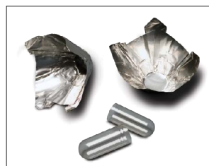
Sample Holder Holds up to 250 mg sample
