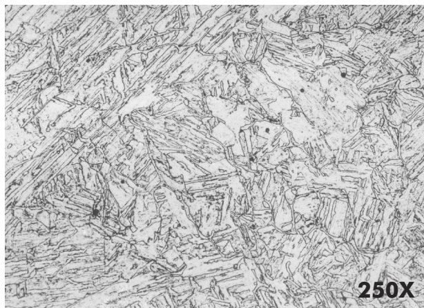
Figure 1. Vilella's reagent—the delta ferrite phase is difficult to detect in the martensitic matrix.
