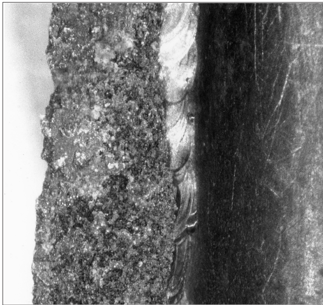
FIGURE 2. Stereo-pair of SAE 1045 tube failure, 4X.
