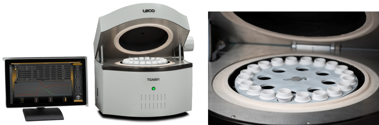
Figure 2: TGA801 open with crucibles – Picture of crucible carousel
