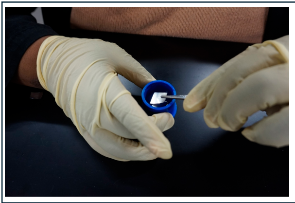
Figure 3. Placing foils on the hardened layer.
